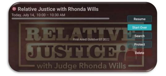
To protect a recorded program from being accidentally deleted choose the Protect option and press OK on your remote. If the recording is protected, highlight and press OK to Unprotect the program from being deleted. You can delete a recorded program by highlighting the Delete option. If you choose to Delete a program, you will receive a prompt asking you to Delete Recording, highlight Delete and press OK.
